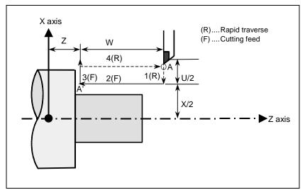
Fig. 4.1.1.1 (a) Straight cutting cycle
