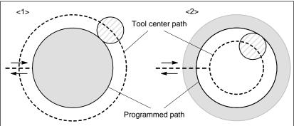
Fig. 5.3 (d) Tool center paths when positive and negative cutter compensation values are specified
