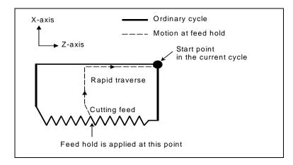
The angle of chamfering during retraction is the same as that of chamfering at the end point.
