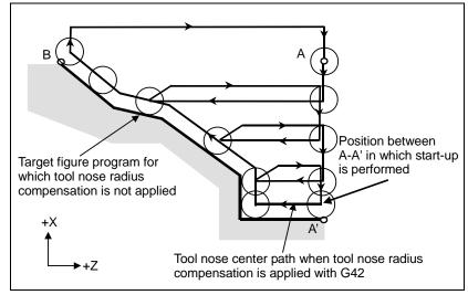
Fig. 6.4.1 (r) Path when tool nose radius compensation is applied
