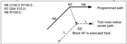
In offset mode, the number of blocks without movement consecutively specified must not exceed N-2 (where N is the number of blocks to read in offset mode (parameter No. 19625). If commanded, a vector whose length is equal to the offset value is produced in a normal direction to tool motion in earlier block, so overcutting may result.
