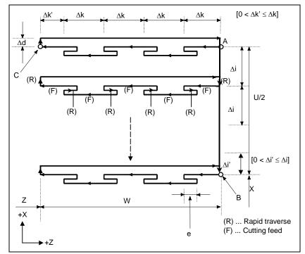
Fig. 4.2.5 (a) Cutting path in end face peek drilling cycle
