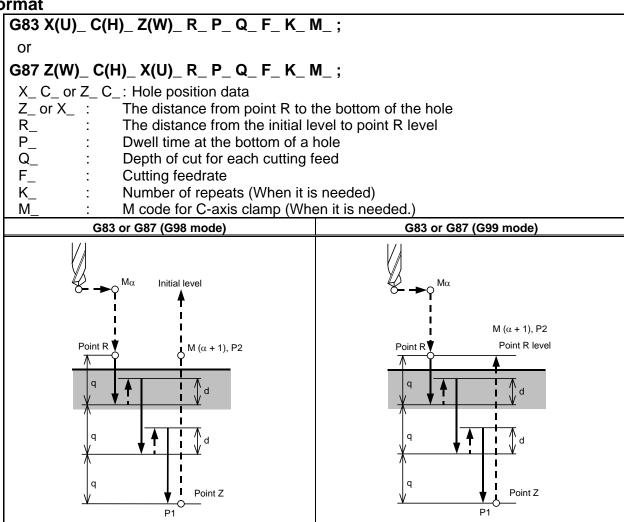
$M\alpha$ : M code for C-axis clamp  $M(\alpha + 1)$ : M code for C-axis unclamp P1 : Dwell specified in the program Dwell specified in parameter No. 5111 P2 :
