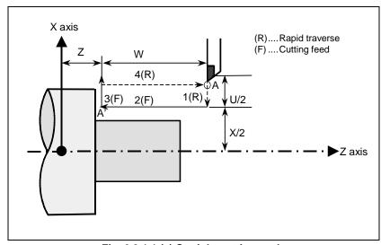
Fig. 6.3.1.1 (a) Straight cutting cycle
