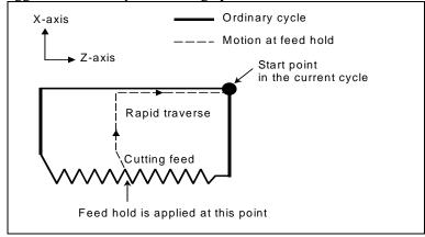
The angle of chamfering during retraction is the same as that of chamfering at the end point.
