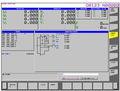
Fig. 2.1.9 (c) Chuck barrier setting screen (15-inch display unit)
