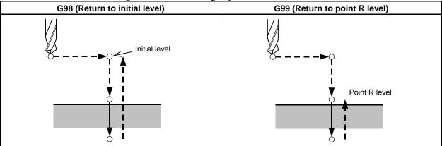
Fig. 6.5 (b) Initial level and point R level
