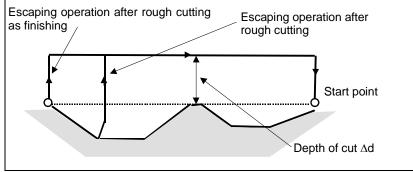
Fig. 6.4.1 (I) Escaping operation when the tool returns to the start point (type II)
