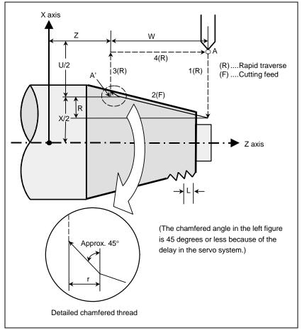
Fig. 4.1.2.2 (a) Taper threading cycle
