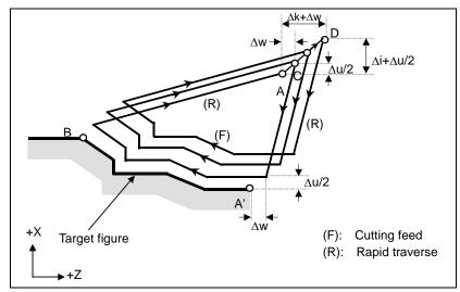
Fig. 6.4.3 (c) Cutting path in pattern repeating
