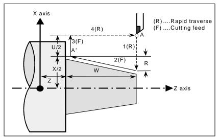
Fig. 4.1.1.2 (a) Taper cutting cycle
