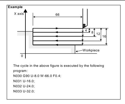
The modal values common to canned cycles are cleared when a one-shot G code other than G04 is specified.
