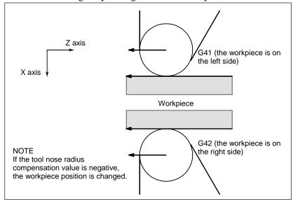
Fig. 5.2.4 (b) When the workpiece position is changed
