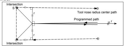
Also in case of arc to straight line, straight line to arc and arc to arc, the reader should infer in the same procedure.
