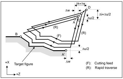
Fig. 4.2.3 (t) Cutting path in pattern repeating
