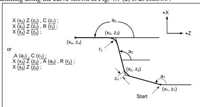
Fig. 4.9 (a) Machining Drawing (example)
