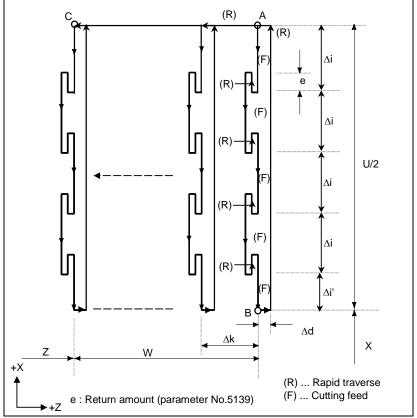
Fig. 6.4.6 (a) Outer diameter/internal diameter drilling cycle
