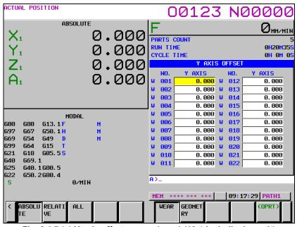
Fig. 2.1.7 (g) Y-axis offset screen (wear) (10.4-inch display unit)
