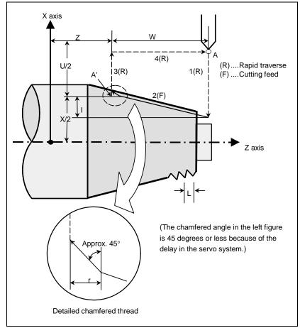
Fig. 6.3.2.2 (a) Taper threading cycle
