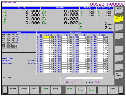
Fig. 2.1.7 (k) Y-axis offset screen (tool geometry)(15-inch display unit)
