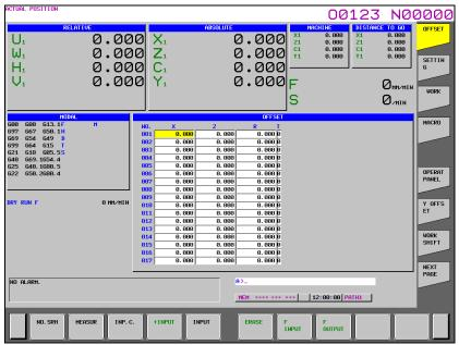
Fig. 2.1.4 (b) Tool offset screen (15-inch display unit)
