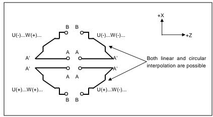
Fig. 4.2.2 (s) Signs of the values specified at U and W in stock removal in facing
