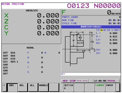
Fig. 2.1.9 (a) Chuck barrier setting screen (10.4-inch display unit)
