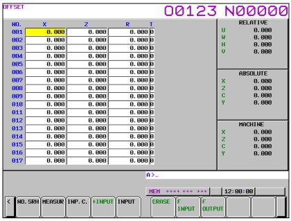
Fig. 2.1.1 (a) Without tool geometry/wear offset (10.4-inch display unit)
