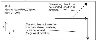
Fig. 4.7 (b) Example of machining which causes alarm PS0051
