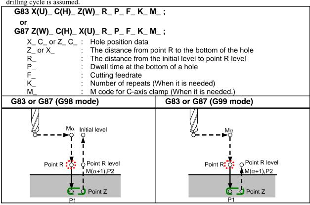
$M\alpha$ M code for C-axis clamp M code for C-axis unclamp  $M(\alpha+1)$ Dwell specified in the program P2 Dwell specified in parameter No. 5111
