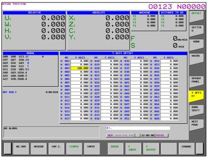
Fig. 2.1.7 (f) Y-axis offset screen (input)(15-inch display unit)
