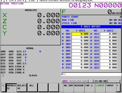
Fig. 2.1.7 (a) Y-axis offset screen (10.4-inch display unit)
