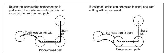
Fig. 5.2.1 (c) Tool path when programming using the tool nose center
