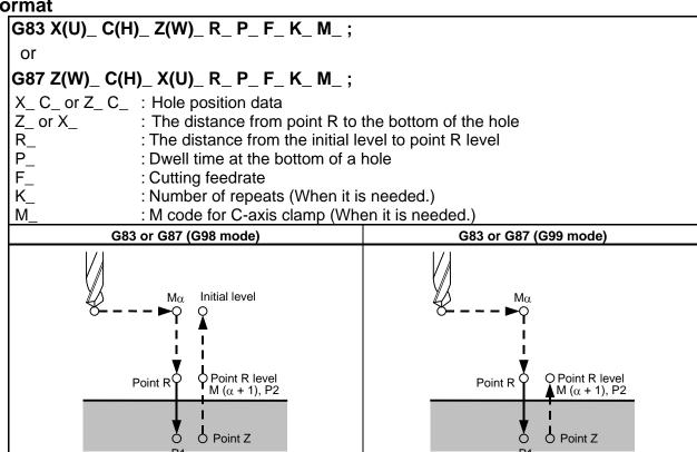
$M\alpha \ :$ M code for C-axis clamp  $M(\alpha + 1)$ : M code for C-axis unclamp Dwell specified in the program P1 P2 Dwell specified in parameter No. 5111
