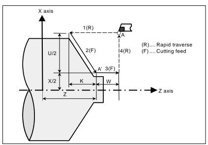
Fig. 6.3.3.2 (a) Taper cutting cycle
