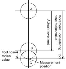
The tool actually moves from point A to point B, but the tool offset value is determined assuming that the tool moves to point C considering the tool nose radius value.
