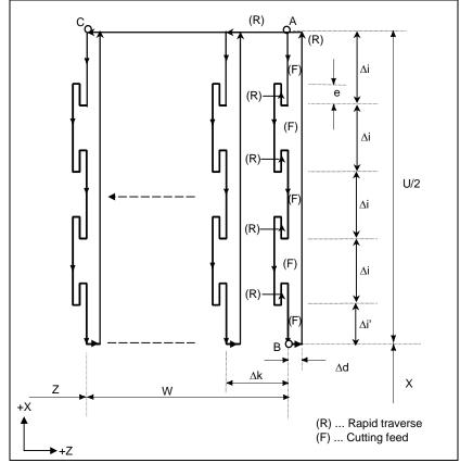
Fig. 4.2.6 (b) Outer diameter/internal diameter drilling cycle
