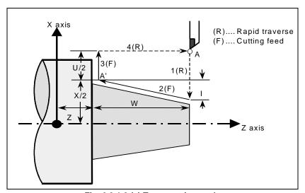
Fig. 6.3.1.2 (a) Taper cutting cycle
