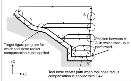
Fig. 4.2.1 (q) Path when tool nose radius compensation is applied
