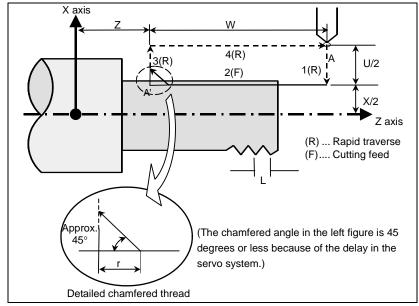
Fig. 6.3.2.1 (a) Straight threading
