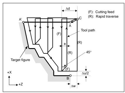
Fig. 4.2.2 (r) Cutting path in stock removal in facing (type I)
