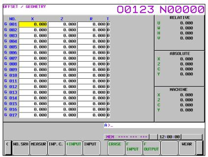
Fig. 2.1.1 (b) With tool geometry offset (10.4-inch display unit)
