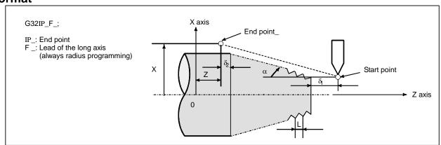
Fig. 3.1 (b) Example of threading
