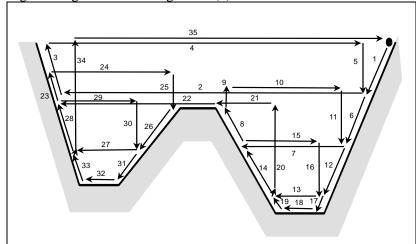
Fig. 6.4.1 (o) Cutting path for multiple pockets (type II)
