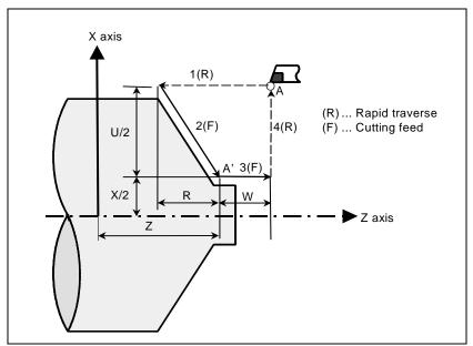
Fig. 4.1.3.2 (a) Taper cutting cycle
