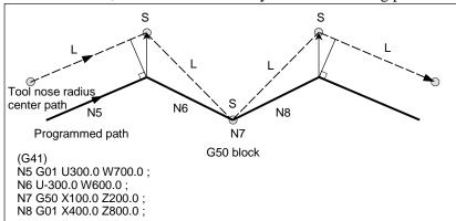
Before specifying G28 (reference position return), G29 (return from reference position), G30 (second, third, and fourth reference position returns), G30.1 (floating reference position return), and G53 (machine coordinate system selection) commands, cancel offset mode, using G40. If an attempt is made to specify any of the commands in offset mode, the offset vector temporarily disappears.
