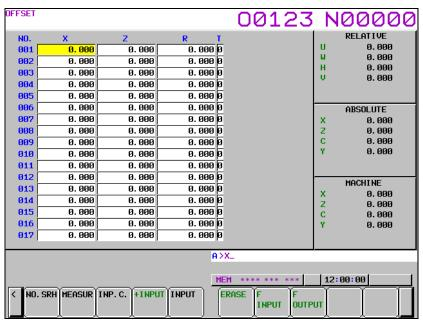
Fig. 2.1.4 (a) Tool offset screen (10.4-inch display unit)
