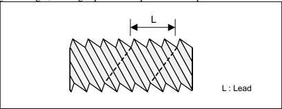
Fig. 3.3 (a) Multiple thread screws.
