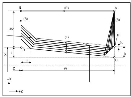
Fig. 4.2.7 (a) Cutting path in multiple threading cycle
