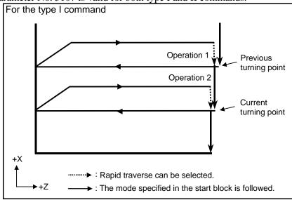
For the type I G71 and G72 commands, operations 1 and 2 to the current turning start point that are usually performed in 2 cycles can be performed in 1 cycle by setting bit 1 (ASC) of parameter No. 5107 to 1. The feed mode specified in the start block in the program for a target figure (G00 or G01) is used. Bit 1 (ASC) of parameter No. 5107 is valid only for the type I command.
