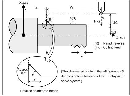
Fig. 4.1.2.1 (a) Straight threading
