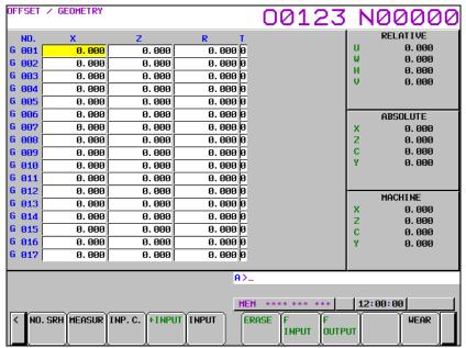
Fig. 2.1.2 (b) Tool offset screen (10.4-inch display unit)
