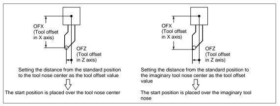
Fig. 5.2.1 (b) Tool offset value when the turret center is placed over the start point
