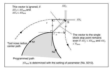
If the vectors are not judged to almost coincide (therefore, are not erased), movement to turn around the corner is performed. The corner movement that precedes the single block stop point belongs to the previous block, while the corner movement that succeeds the single block stop point belongs to the latter block.
