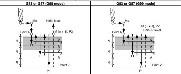
$M\alpha$ : M code for C-axis clamp M code for C-axis unclamp  $M(\alpha + 1)$ : P1 : Dwell specified in the program
