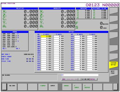
Fig. 2.1.8 (d) 4th/5th axis offset screen (without tool geometry/wear offset) (15-inch display unit)
