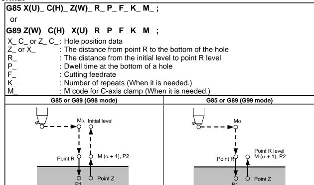
$M\alpha$ : M code for C-axis clamp  $M(\alpha + 1)$ : M code for C-axis unclamp P1: Dwell specified in the program P2: Dwell specified in parameter No. 5111
