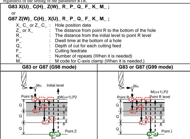
: M code for C-axis clamp Μα  $M(\alpha+1)$ : M code for C-axis unclamp P1 Dwell specified in the program Dwell specified in parameter No. 5111 P2
