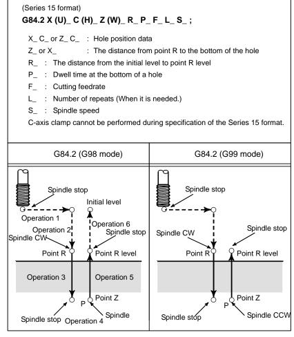
A G code cannot discriminate between front face tapping cycle and side face tapping cycle using Series 15 format commands(G84.2). The drilling axis is determined by plane selection (G17/G18/G19). Specify the plane selection that becomes equivalent to front face tapping cycle or side face tapping cycle as appropriate. (When FXY (bit 0 of parameter No. 5101) is 0, the Z-axis is used as the drilling axis. When FXY is 1, plane selection is as Table 4.5.1 (a).)
