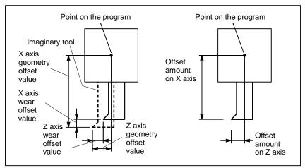
Fig. 5.1.1 (a) If tool geometry offset and tool wear offset are distinguished from each other (left) and if they are not (right)
