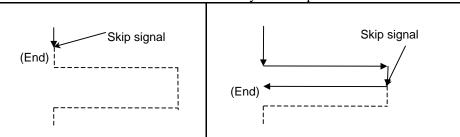
• If the skip signal is input during operation <2> or <5> (dwell), dwell operation is immediately stopped to return to coordinate  $\alpha$  selected as the cycle start point.
