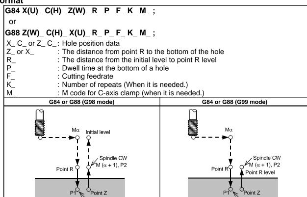
$M\alpha$ : M code for C-axis clamp M ( $\alpha$  + 1): M code for C-axis unclamp P1: D well specified in the program P2: D well specified in parameter No. 5111
