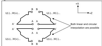
Fig. 6.4.2 (b) Signs of the values specified at U and W in stock removal in facing
