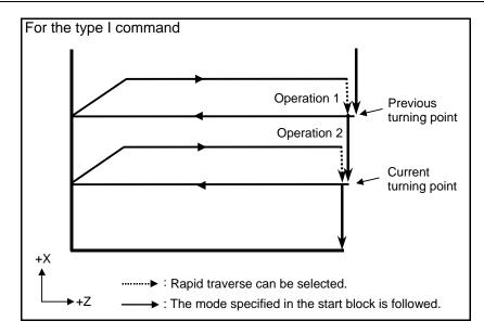
For the type I G71 and G72 commands, operations 1 and 2 to the current turning start point that are usually performed in 2 cycles can be performed in 1 cycle by setting bit 1 (ASC) of parameter No. 5107 to 1. The feed mode specified in the start block in the program for a target figure (G00 or G01) is used. Bit 1 (ASC) of parameter No. 5107 is valid only for the type I command.
