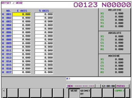
Fig. 2.1.8 (b) 4th/5th axis offset screen (with tool geometry/wear offset) (10.4inch)
