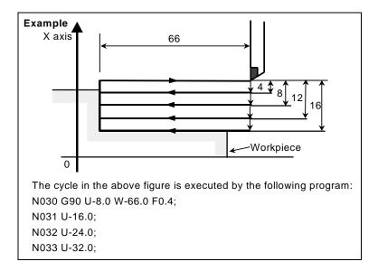
The modal values common to canned cycles are cleared when a one-shot G code other than G04 is specified.
