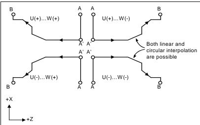
Fig. 6.4.1 (c) Four target figure patterns
