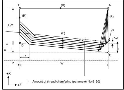
Fig. 6.4.7 (a) Cutting path in multiple threading cycle
