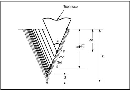
Fig. 4.2.7 (b) Detail of cutting
